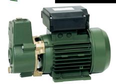
Self-priming peripheral pump with star impeller, with a great suction capacity. Cast iron body with brass ring. Motor support and impeller in brass to avoid the risk of blocking. Driving shaft in stainless steel. Carbon/ceramic mechanical seal.
