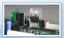
3. Built-in brake resistor, realize frequent acceleration and deceleration freely (optional).
