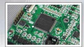
1. Adopting Taiwan DSP to be the core control chip to realize the high speed performance control.
